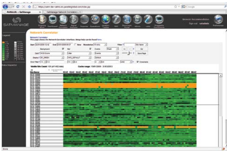
The SatManage network correlator module shows network events relating to Mean Opinion Score and jitter at 15 minute intervals over a 24h period
