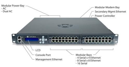
**Uplogix' flagship Local Manager (LM)**, the Uplogix 3200 is available in 8-, 16-, 24- or 32-port models. The Uplogix 3200 is a scalable and robust LM for enterprises that locally manage an ever-growing infrastructure of distributed networking gear, servers and other IT devices located at remote sites, branch locations and data centers.
