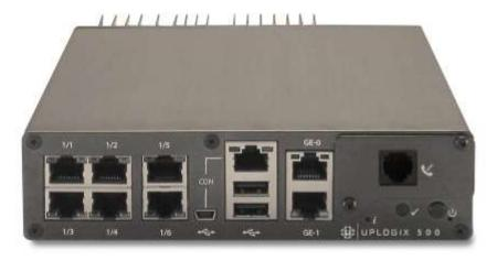
There are six serial ports that can be connected to managed devices including an intelligent power controller.
