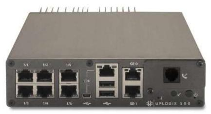
There are six serial ports that can be connected to managed devices including an intelligent power controller.
