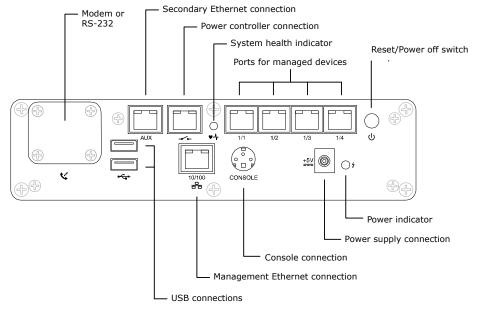
There are five serial ports that can be connected to managed devices, where one port is dedicated for connection to an intelligent power controller.
