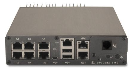
There are six serial ports that can be connected to managed devices, where one port is dedicated for connection to an intelligent power controller.
