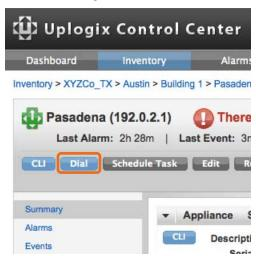
The Control Center Dial applet connects to the modem server with the information preprogrammed in the RAS section of the Local Manager Modem configuration.
