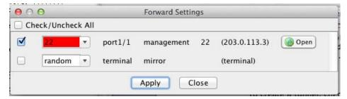
If the drop-down menu turns red, this indicates the local port was unavailable and the tunnel was not created. Choose a different local port that is not currently in use.
