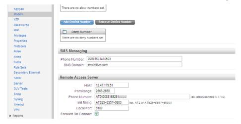
Once the access server information has been configured (in the Remote Access Server section), a blue Dial button appears in the Control Center. Click the Dial button to connect to the Local Manager via out-of-band, circuit switched phone number.
