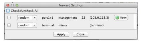
In this example, the Uplogix device has already been configured to forward traffic to port 22 at the management IP address for the device on port 1/2. The screen above allows you to select which tunnels to create. On a device with multiple forwards configured, the above list would be longer.
