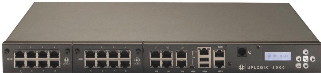
Each expansion bay can be used to add either 4, 8 or 16 serial ports or eight dedicated Ethernet ports, for pairing with serial ports, when direct Ethernet connections are needed for managed devices.
